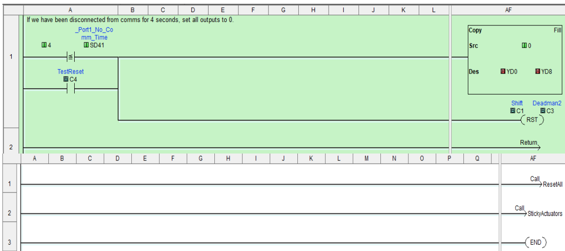
Figure 9: Security of SHIFT and Deadman Switch by using Reset All block for resetting the system if servers are disconnected for 4 seconds
